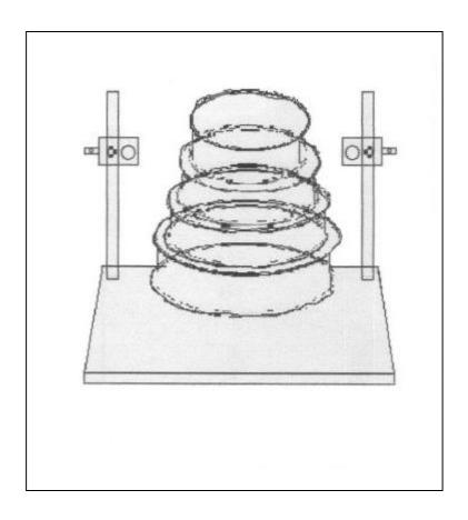
FO-BLA Model is a JAIN LASERTECH make F.O. Bending Loss Apparatus that is available as part of a set of extra accessories that can be used with our standard Diode Laser Characterization Kit.
