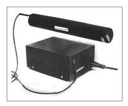
For **cylindrical** laserheads (where powersupply is seperate), kinematic mount is avalable as option. Otherwise, choose **Self-contained** models as shown in the photograph at right. Further, besides Green, other models are available in Red, Yellow and Orage colours. They serve as low cost sources of well-defined monochromatic wavelengths so very useful for studying characteristics of optical elements and materials using either the reflective or the transmissive properties.
