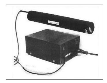
Model VDL-30 is 3 mW, Model VDL-100 is 10 mW and Model VDL-200 is 20 mW. Matched **stand mounted kinematic holders** are available as option for convenient beam positioning and alignment.
