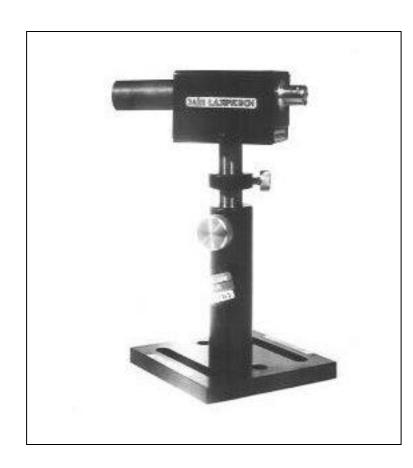
PD-10 Model is a JAIN LASERTECH make Mounted Photo Detector that exhibits a highly linear responsivity over a vide spectral range allowing accurate detection of very low levels across the visible and into the near-IR.
